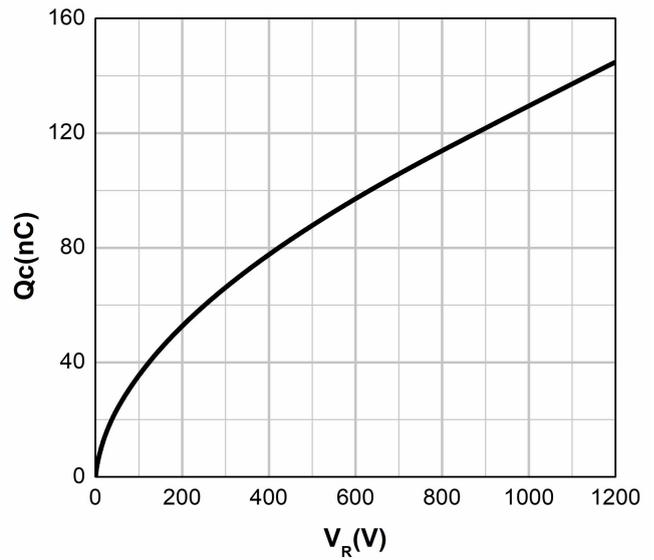
Figure 4. Total Capacitance Charge vs. Reverse Voltage
