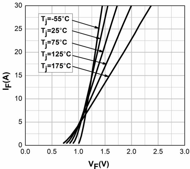
Figure 1. Forward Characteristics
