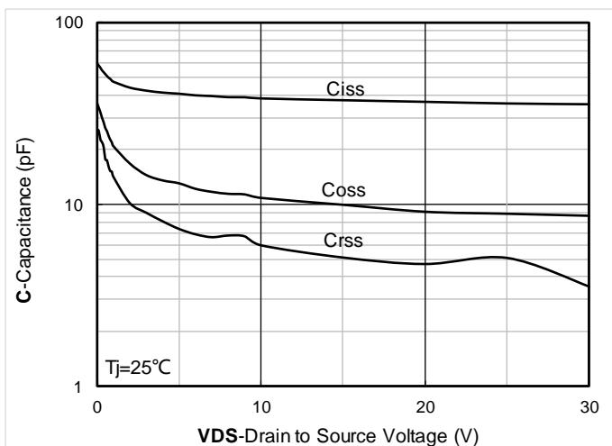
Figure 3. Capacitance Characteristics
