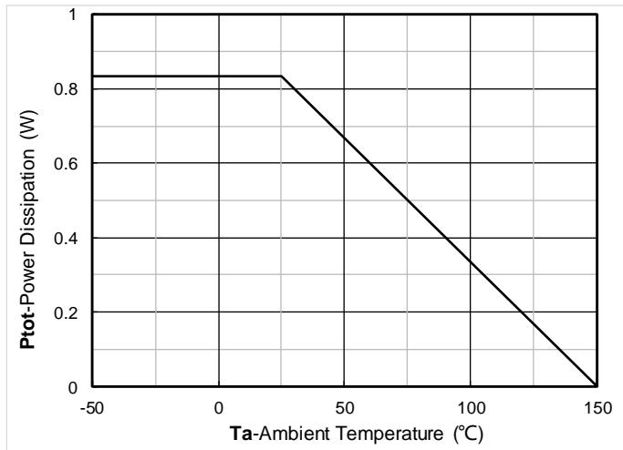
Figure 12. Power dissipation
