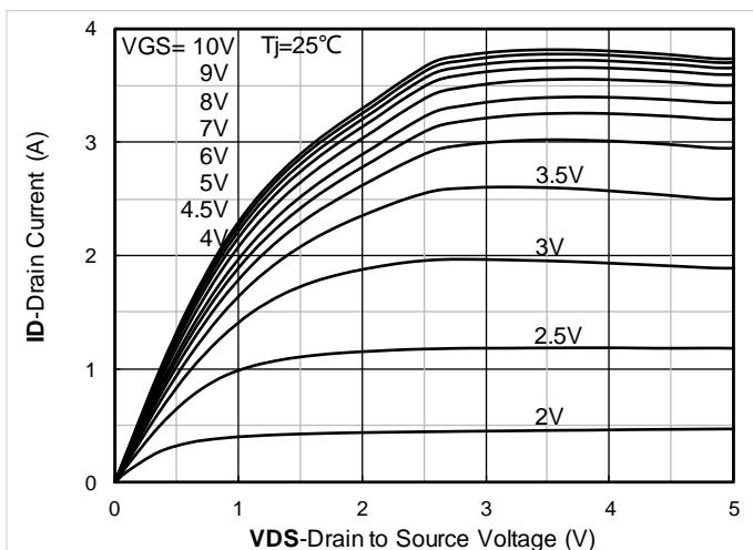
Figure 1. Output Characteristics
