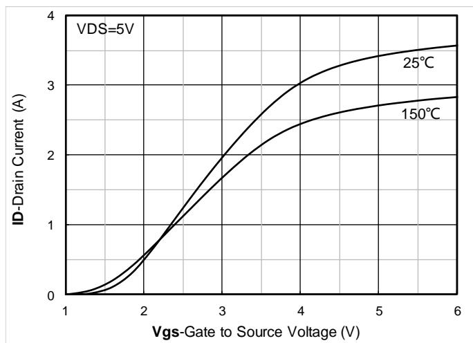
Figure 2. Transfer Characteristics
