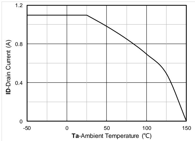
Figure 11. Current dissipation
